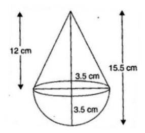
Total height of the toy = 15.5 cm  $\therefore$  Height of the cone = 15.5 - 3.5 = 12 cm Slant height of the cone =  $\sqrt{(3.5)^2 + (12)^2}$ =  $\sqrt{12.25 + 144}$ =  $\sqrt{156.25} = 12.5$  cm  $\therefore$  TSA of the toy = CSA of hemisphere + CSA of cone =  $2\pi r^2 + \pi r l$ =  $2\pi (3.5)^2 + \pi (3.5)(12.5)$ =  $24.5\pi + 43.75\pi = 68.25\pi$ =  $68.25 \times \frac{22}{7} = 214.5$  cm<sup>2</sup>
